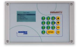
Remote management using "Agronic App", SMS messages, as well as PC connections to three users or to an Irrigation Community software.
